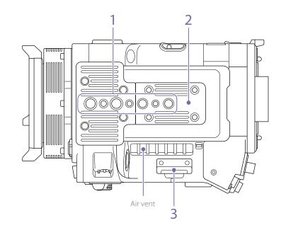
1. Tripod plate attachment holes
