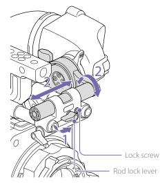
3 Tighten the rod lock lever.
