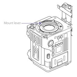
2 Place the PL lens adaptor back in its original position, insert the six hex screws (2.5 mm), and tighten the screws to a tightening torque of 0.8 ± 0.12 N·m using a hex wrench (2.5 mm).
