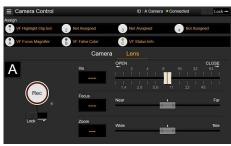
Lens controls for zoom, focus, and iris are displayed on the Lens screen.
