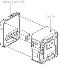
3 Attach the AXS-R7 to the unit, and tighten the four hex screws.
