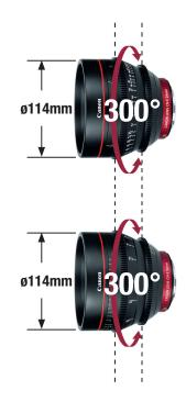
Uniform Front Lens Diameters and Gear Positions on Focus and Iris Rings, as well as 300° of Smooth Rotation on Focus Ring.
