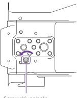
Screwdriver hole (with cap removed)
