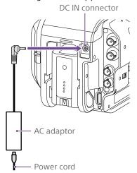
Connect the AC adaptor to the DC IN connector on the camcorder, and connect the power cord (supplied) to an AC power source.
