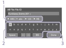
Press the arrow buttons or turn the multifunction dial to select a character type, then apply the setting.
