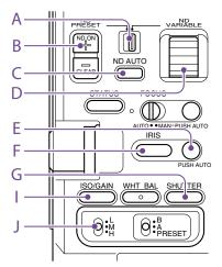
You can adjust the brightness by adjusting the iris, gain, shutter speed, and by adjusting the light level using ND filters. You can also make adjustments automatically.
