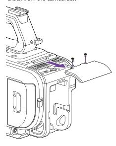
Align the protrusions of the XDCA-FX9 with the left and right grooves of the camcorder and slide it all the way in and then down into the connector block.
