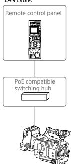
7 Turn the unit on. The unit enters remote control mode, allowing shooting operations of the unit to be controlled by the remote control panel.
