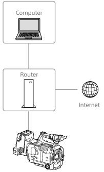
Connect to the Internet router as described in "Connecting to a Device using a LAN Cable" (page 60).
