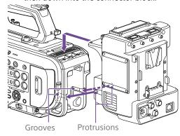
Tighten the two screws on the top of the XDCA-FX9 to secure the XDCA-FX9.
