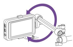
If the viewfinder is turned 180° as shown in the following diagram, set the MIRROR switch to the ROT position to flip the image display and text display horizontally and vertically.
