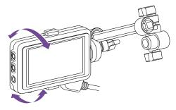
You can adjust the angle so that the viewfinder is facing the subject. Setting the MIRROR switch to the B/T position flips the left and rights sides of the image on the LCD screen, but the image is recorded in the correct orientation.
