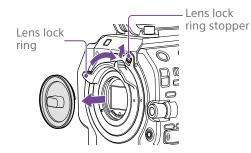
Align the lens mount mark (white) with the camcorder, carefully insert the lens, and slowly turn the lens lock ring counterclockwise to secure the lens.
