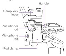
Adjust the left/right positioning of the viewfinder, tighten the clamp lever, connect the viewfinder cable to the viewfinder connector of the camcorder, and secure the viewfinder cable in the cable clamper.
